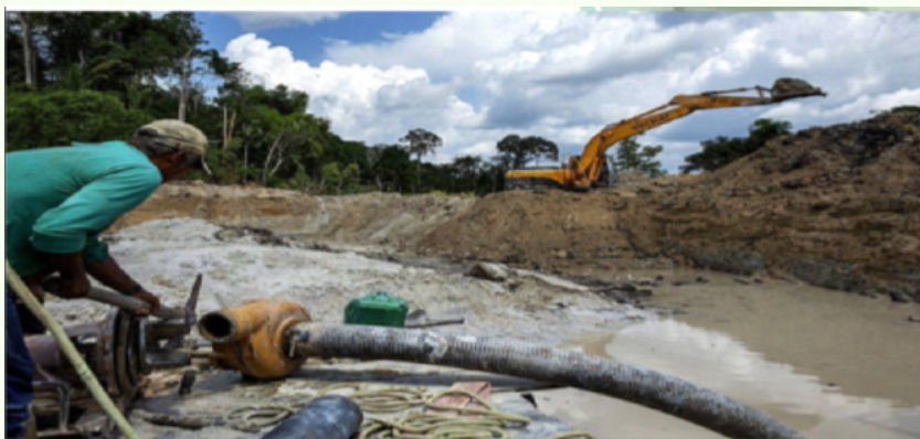
Image 3 - Illegal mining activity on indigenous lands in the Das Tropas river tributary of the Tapajós river, use of machines coupled to water hoses called “Tatuzão”..
