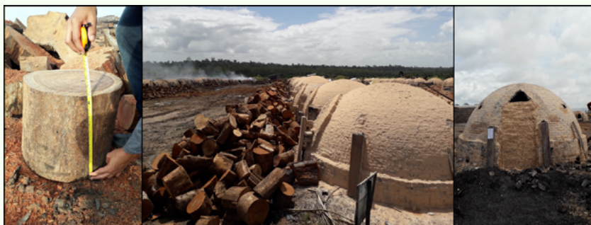
Figure 2. Process of production of charcoal in Rio Capim farm. Source: Author (2019)
